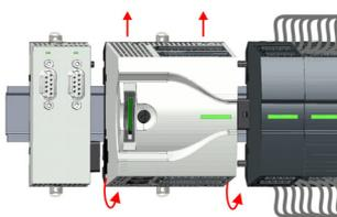
3. → Remove the CPU with a rotation upwards from the profile rail.
