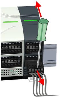
4. → In this way, remove all plugged connectors on the periphery module.
