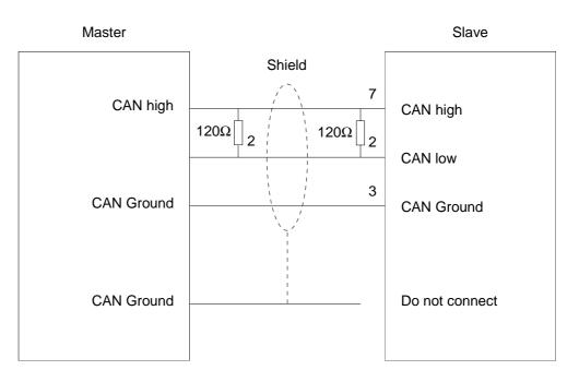
**Line termination** All stations on systems having more than two stations are wired in parallel. This means that the bus cable must be looped from station to station without interruptions.
