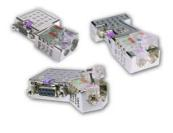
Via the order number VIPA 972-0DP10 you may order the bus connector "EasyConn". This is a bus connector with switchable terminating resistor and integrated bus diagnostic.
