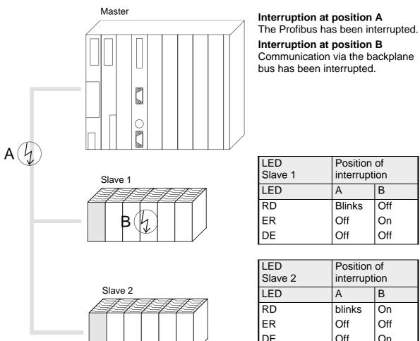
LED Position of Slave 1 interruption LED Α В Blinks Off Off On Off Off
