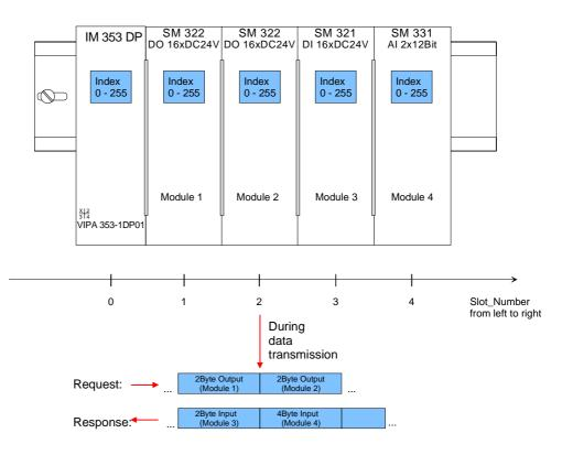
Each data block can be up to 244Bytes. In the case of modular devices, the slot number is assigned to the modules. Compact devices are regarded as a unit of virtual modules. These can also be addressed whit slot number and index. Through the length specification in the read/write request, it is also possible to read/write parts of a data block.
