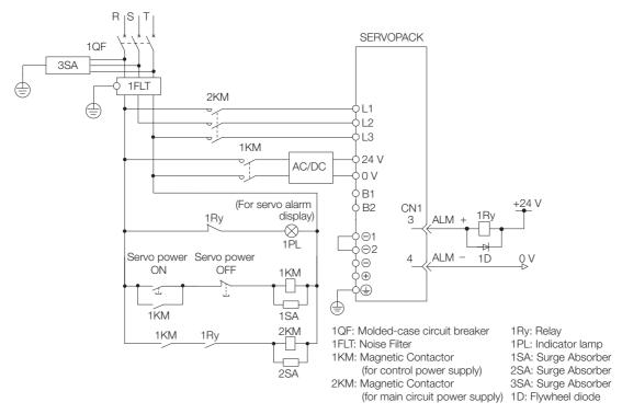
4.3.4 Power Supply Wiring Diagrams
