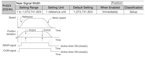
Note: Normally, set Pn524 to a value that is larger than the setting of Pn522 (Positioning Completed Width).
