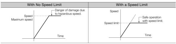
Note: The actual limit of Servomotor speed depends on the load conditions on the Servomotor.
