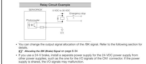
4.4.4 Wiring the SERVOPACK to the Holding Brake
