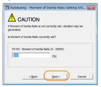
**9.** First confirm safety around moving parts. Turn ON the servo, enter a reference from the host controller, and then click the **Start tuning** Button.
