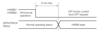
Note: 1. The OFF status is not recognized if the OFF interval of the /HWBB1 or /HWBB2 signal is 0.5 ms or shorter. 2. You can check the status of the input signals by using monitor displays.
