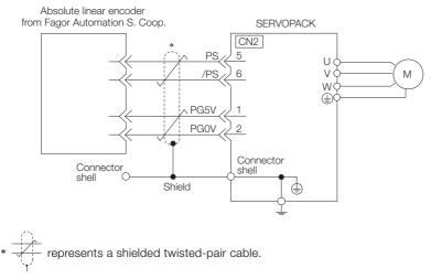
4.4.3 Wiring the SERVOPACK to the Encoder
