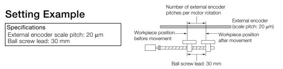
If the external encoder is connected directly to the Servomotor, the setting will be 1,500 (30 mm/0.02 mm = 1,500).
