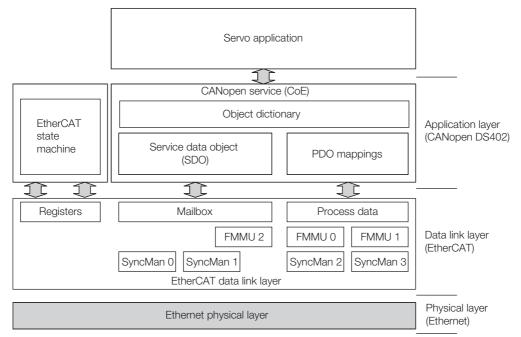
The object dictionary in the application layer includes parameters, application data, and PDO mapping information between the master and slaves.
