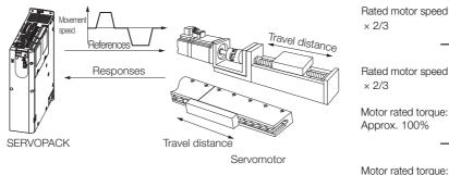
x 2/3 Rated motor speed x 2/3 Motor rated torque: Approx. 100% Example of Automatic Operation Pattern
