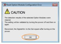
7. Turn the power supply to the SERVOPACK OFF and ON again.
