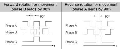
Note: The pulse width of encoder phase C depends on the setting of Pn212 (Number of Encoder Output Pulses) or Pn281 (Encoder Output Resolution). It is the same as the width of phase A. Even for Pn000 = n.DDD1 (reverse operation), the output phase form is the same as shown above.
