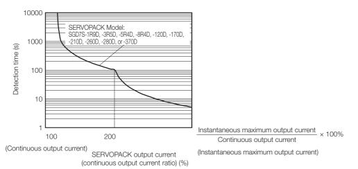
Note: The above overload protection characteristics do not mean that you can perform continuous duty operation with an output of 100% or higher.
