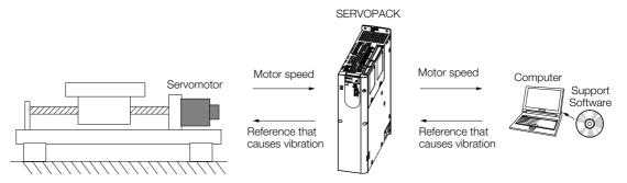
The Servomotor is used to cause machine vibration and then the speed frequency characteristics for the motor torque are measured. The measured frequency characteristics can be used to determine the machine resonance.
