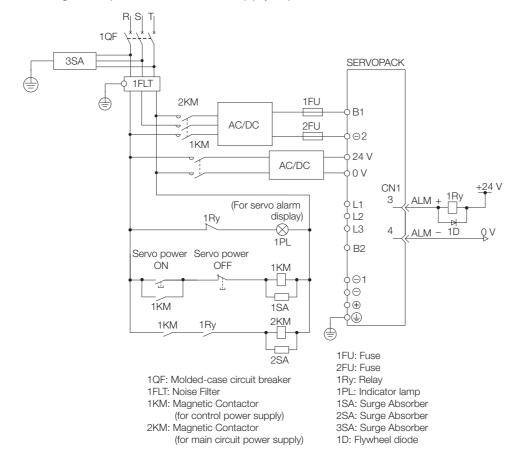
4.3.4 Power Supply Wiring Diagrams
