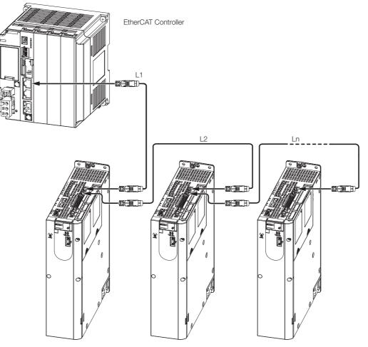
Note: The length of the cable between stations (L1, L2,  $\dots$  Ln) must be 50 m or less.
