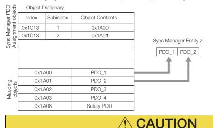
• The PDO mapping objects (indexes 1600h to 1603h, 1608h, 1A00h to 1A03h, and 1A08h) and the Sync Manager PDO assignment objects (index 1C12h and 1C13h) can be written only in Pre-Operation state.
