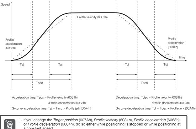
or Profile deceleration (6084h), do so either while positioning is stopped or while positioning at a constant speed.
