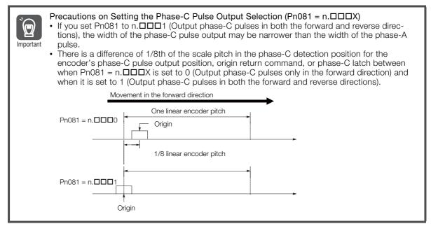
Observe the following precaution if you set Pn081 to n. **DDD** (Output phase-C pulses only in the forward direction).
