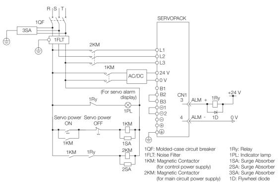
• Wiring Example for Three-Phase, 400-VAC Power Supply Input: SGD7S-210D, -260D, -280D, and -370D
