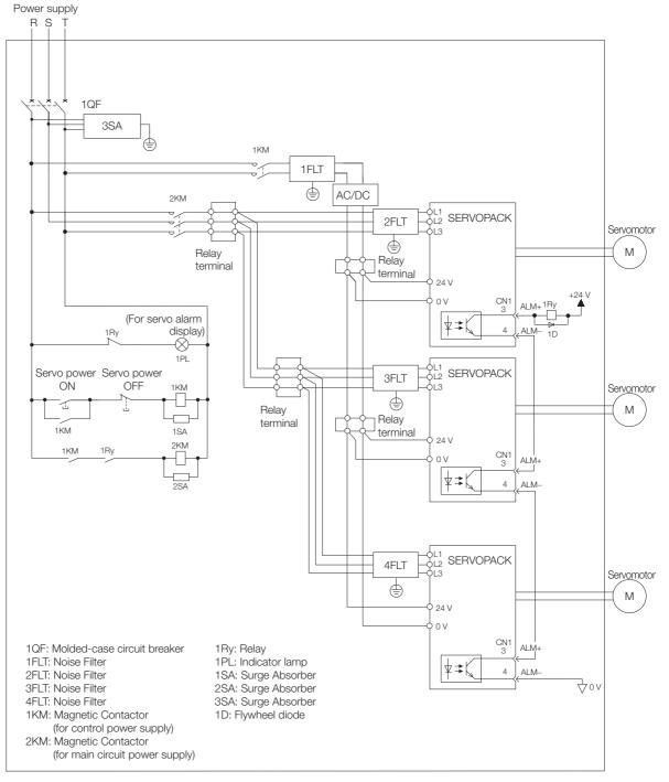
To comply with UL/cUL standards, you must install a branch circuit protective device at the power supply input section to each SERVOPACK. Refer to the following document for details.  $\square \Sigma$ -7-Series  $\Sigma$ -7S and  $\Sigma$ -7W SERVOPACK with 400 V-Input Power Safety Precautions (Manual No.: TOMP C710828 02)
