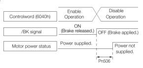
This parameter sets the timing of stopping power supply to the Servomotor while the Servomotor is stopped.
