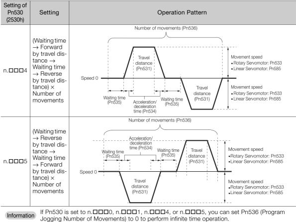
Jogging Number of Movements) to 0 to perform infinite time operation. You cannot use infinite time operation if Pn530 is set to n. DDD2 or n. DDD3. If you perform infinite time operation from the Digital Operator, press the **JOG/SVON** Key to turn OFF the servo to end infinite time operation.
