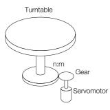
Because the turntable moves in only one direction, the upper limit to the number of rotations that can be counted by an absolute encoder will eventually be exceeded.
