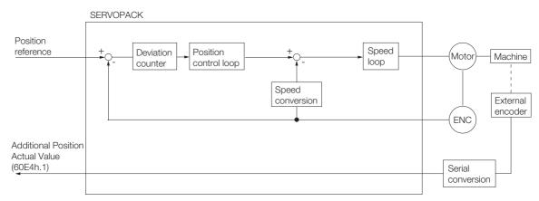
The following block diagram shows monitoring an external encoder in the Profile Position Mode.
