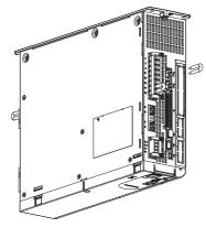
2. Connect the External Regenerative Resistor between the B1 and B2 terminals on the SERVOPACK.
