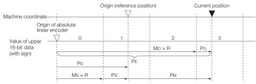
The current position  $P_M$  in the machine coordinate system is calculated as follows:
