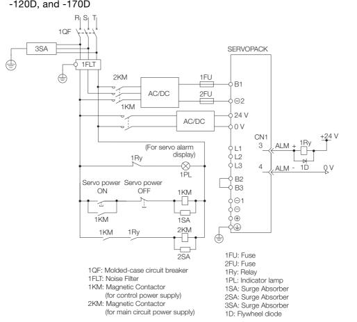
• Wiring Example for DC Power Supply Input: SGD7S-1R9D, -3R5D, -5R4D, -8R4D, -120D, and -170D
