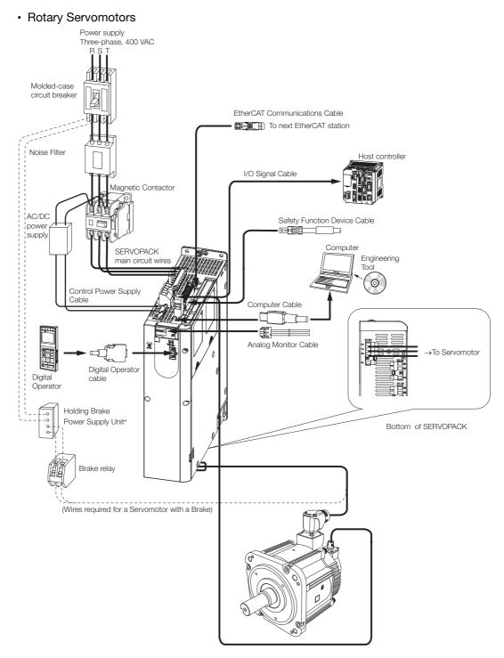
\* The power supply for the holding brake is not provided by Yaskawa. Select a power supply based on the holding brake specifications.
