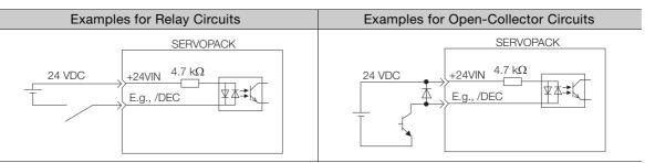
Note: The 24-VDC external power supply capacity must be 50 mA minimum.
