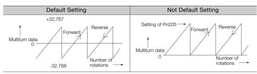
Information When the encoder is set to be used as a single-turn absolute encoder (Pn002 =  $n.\square 2 \square \square$ ), the multiturn data will always be zero. It is not necessary to reset the absolute encoder. Also, an alarm related to the absolute encoder (A.810 or A.820) will not occur.
