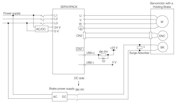
BK-RY: Brake control relay 1D: Flywheel diode
