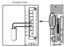
Set Pn600 (Regenerative Resistor Capacity) and Pn603 (Regenerative Resistor Resistance). Refer to the following section for details on the settings.
