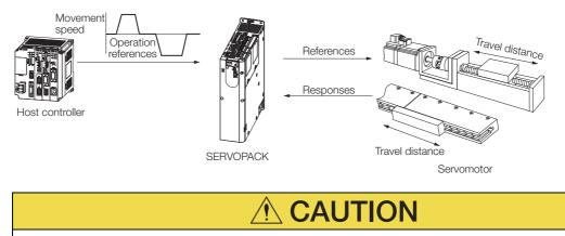
• Because autotuning with a host reference adjusts the SERVOPACK during automatic operation, vibration or overshooting may occur. To ensure safety, make sure that you can perform an emergency stop at any time.
