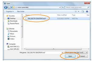
7. Confirm that the motor parameter file information that is displayed is suitable for your Servomotor, and then click the Next Button.
