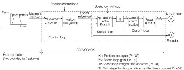
In order to manually tune the servo gains, you must understand the configuration and characteristic of the SERVOPACK and adjust the servo gains individually. In most cases, if you greatly change any one parameter, you must adjust the other parameters again. To check the response characteristic, you must prepare a measuring instrument to monitor the output waveforms from the analog monitor.
