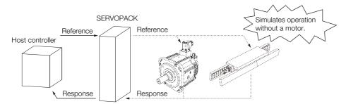
Use  $Pn00C = n.\square\square\squareX$  to enable or disable the test without a motor.
