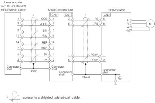
4.4.3 Wiring the SERVOPACK to the Encoder
