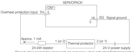
Closed when normal (low temperature) and open when activated (high temperature)
