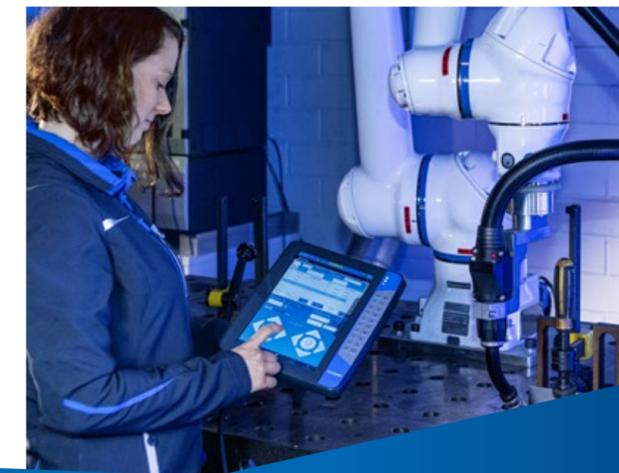
Use the Direct Teach buttons, Weld Builder or the Smart Pendant to program **Weld4Me CE**
