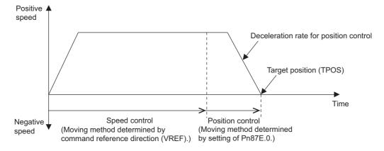
Changing to Position Control in the Reverse Direction (Pn87E.0) of the Direction of Speed Control (Command Reference Direction)
