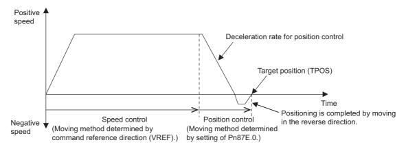
Note: If the Function Switch of Rotational Coordinate System (Pn87E.0) is set to absolute positioning (Pn87E.0 = 0) or to positioning for the shortest path (Pn87E.0 = 3), the moving method will depend on the timing of changing to position control.
