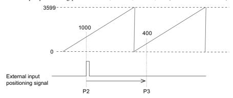
• Conditions: Starting Point of Rotational Coordinate System (Pn87C): 0
