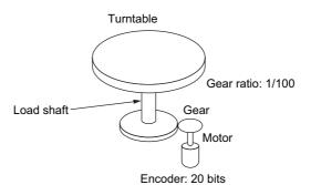
• Conditions: A turntable is controlled with rotational coordinates where one revolution equals 360°, which is equal to 36,000 reference units.
