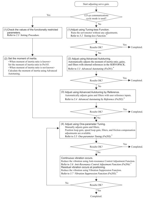
Refer to the Σ-V Series User's Manual Design and Maintenance, MECHATROLINK-III Communications Reference. (No.: SIEP S800000 64/65)
