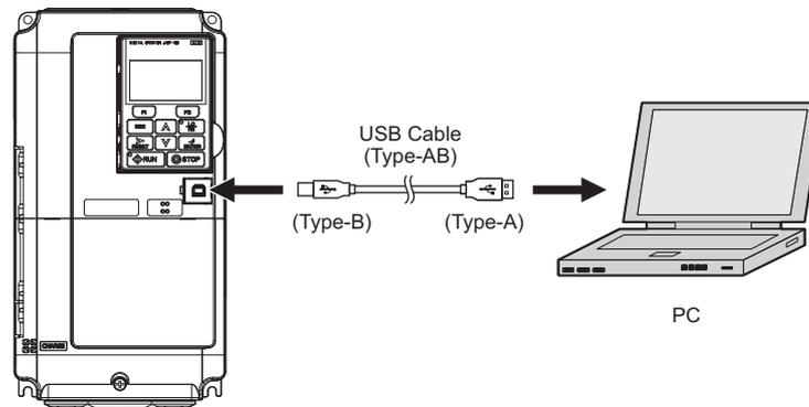
Figure 3.28 Connecting to a PC (USB)
