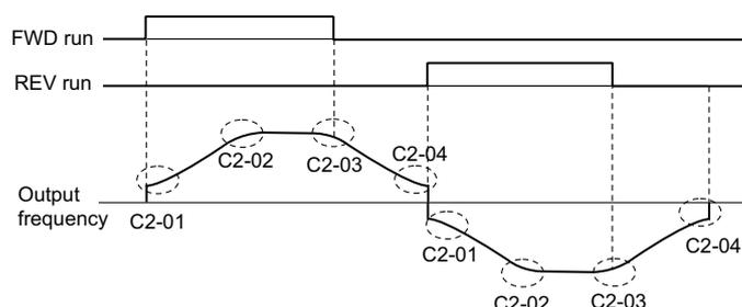
**Figure 5.35 S-Curve Timing Diagram - FWD/REV Operation**
