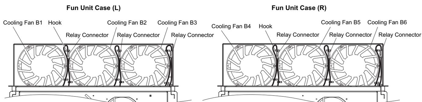
Figure 7.46 Cooling Fan Wiring: Models 4A0930 and 4A1200
