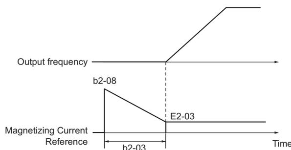
Figure 5.19 Magnetic Flux Compensation
