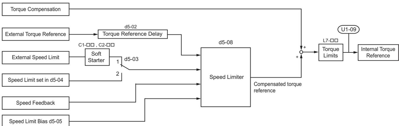
Figure 5.53 Torque Control Block Diagram
