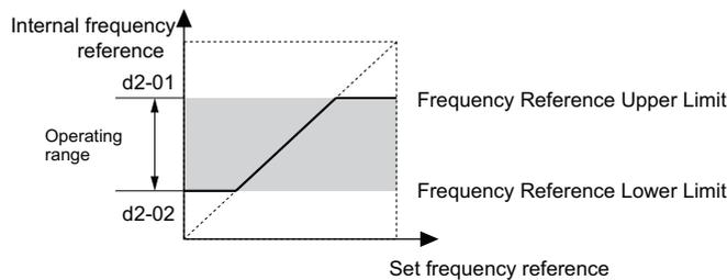
Figure 5.46 Frequency Reference: Upper and Lower Limits
