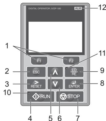
Figure 4.1 Keys and Displays on the Digital Operator
