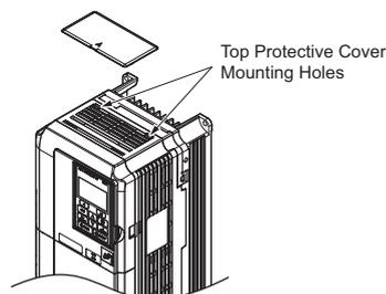
Figure 3.16 Reattaching the Top Protective Cover
