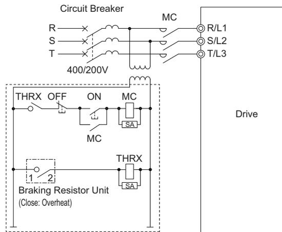
**Figure 8.20** Power Supply Interrupt for Overheat Protection (Example)
