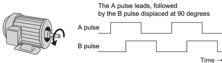
**Figure 8.16 Displacement of A and B Pulses**
