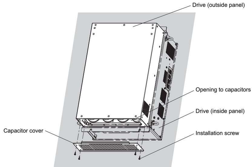
**Figure D.11 Capacitor Cover**
