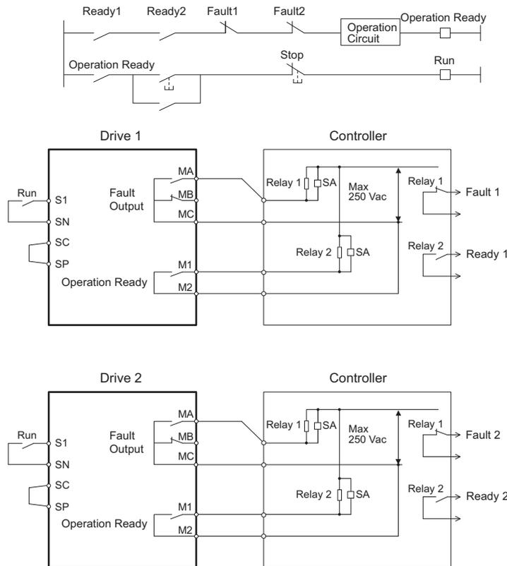
Figure 3.29 Interlock Circuit Example
