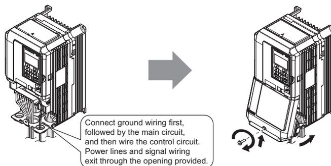
Figure 3.5 Reattaching the Terminal Cover on an IP20/UL Type 1 Enclosure Drive
