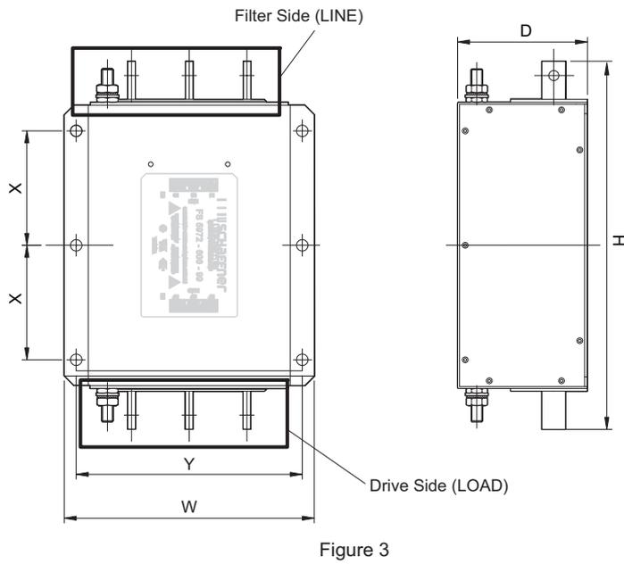
Figure D.7 EMC Filter Dimensions (Manufacturer: Schaffner)
