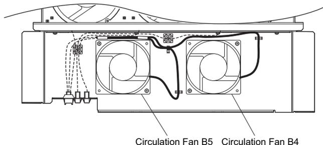
Figure 7.38 Cooling Fan Wiring: 4A0515 and 4A0675
