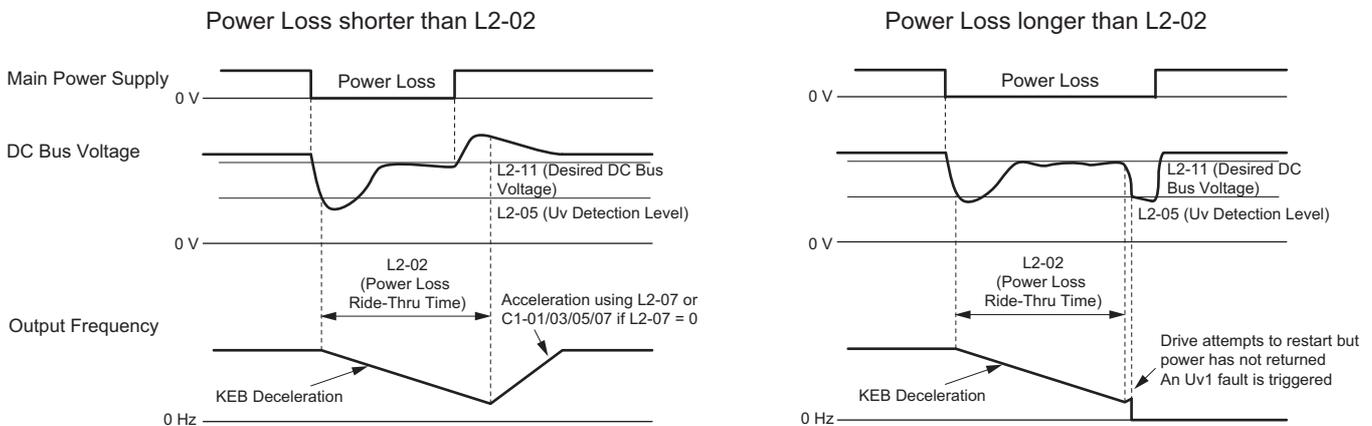
Figure 5.96 KEB Operation Using L2-02, Without KEB Input
