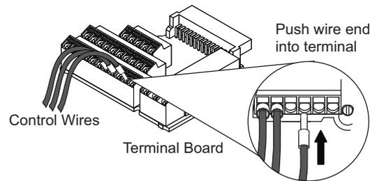
**Figure 3.22 Terminal Board Wiring Guide**
