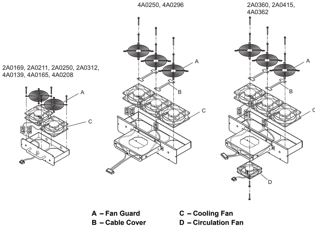
Figure 7.22 Fan Unit Disassembly: 2A0169 to 2A0415, 4A0139 to 4A0362
