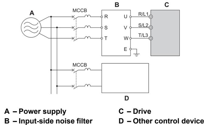
Figure 8.27 Input-Side Noise Filter (Three-Phase 200/400 V)
