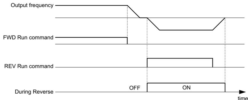
Figure 5.78 Reverse Direction Output Example Time Chart
