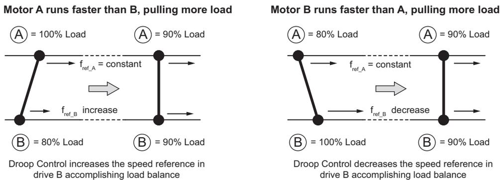
Figure 5.30 Droop Control in a Traverse Application
