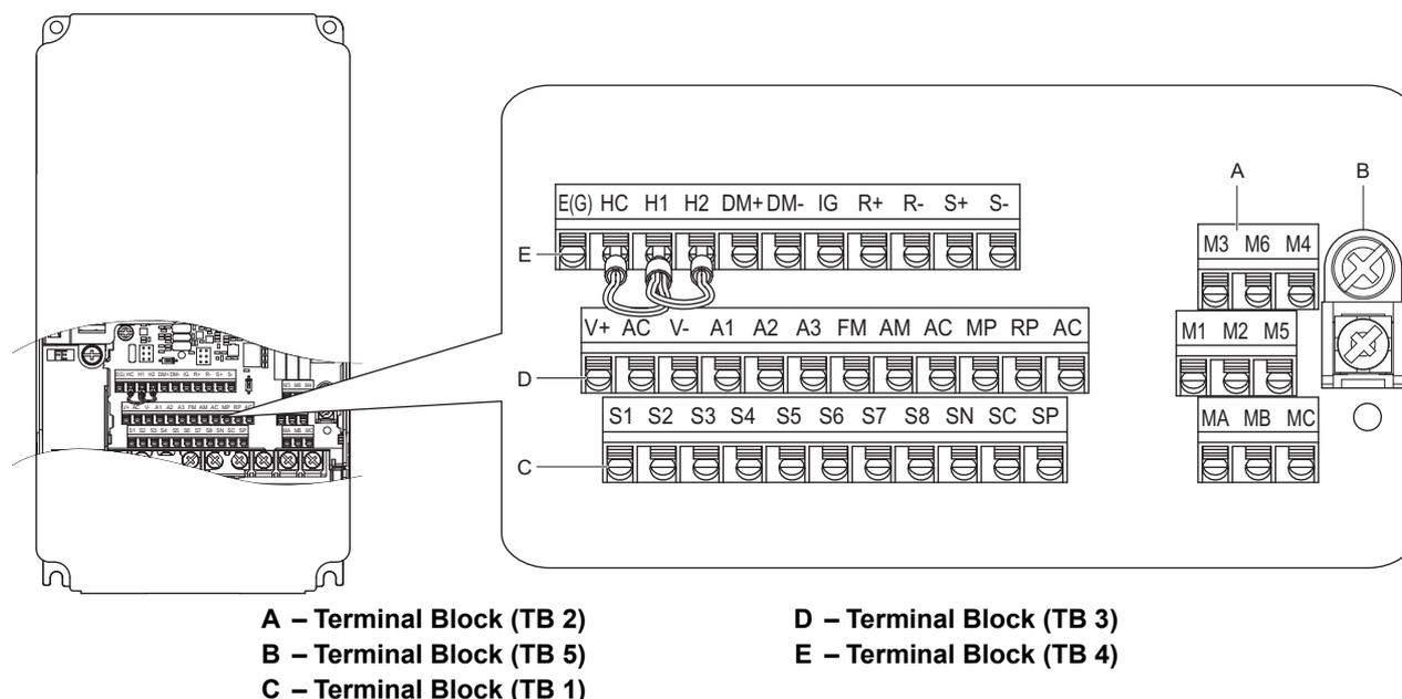
Figure 3.20 Control Circuit Terminal Arrangement
