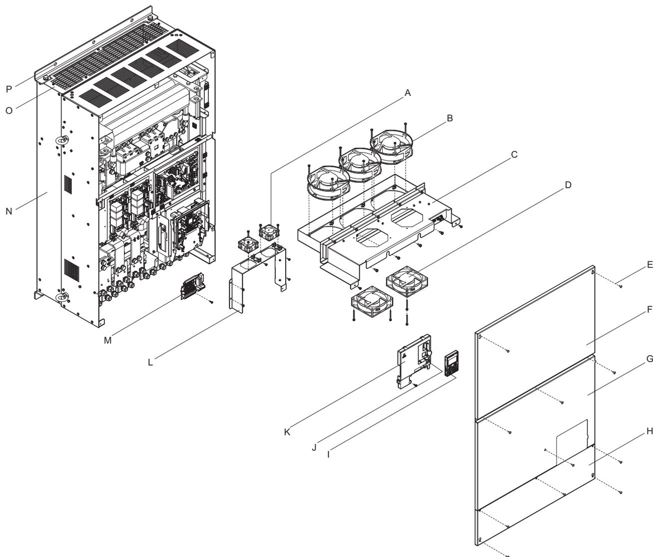
Figure 1.7 Exploded view of IP00 Enclosure Type Components (CIMR-A□4A0515A, 0675A)
