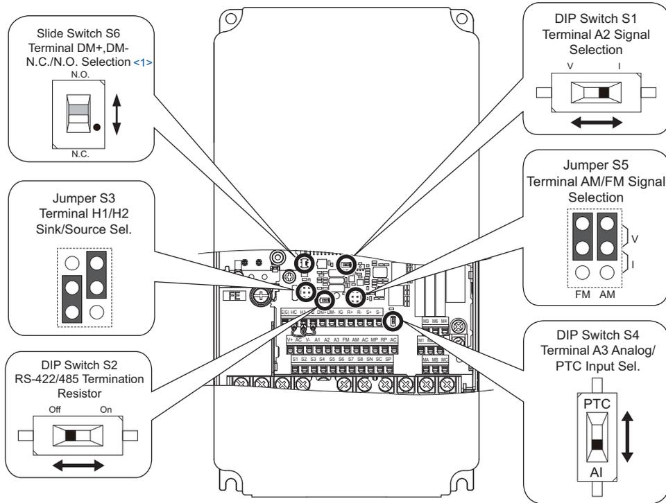
Figure 3.25 Locations of Jumpers and Switches on the Terminal Board
