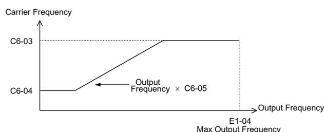
Figure 5.43 Carrier Frequency Changes Relative to Output Frequency
