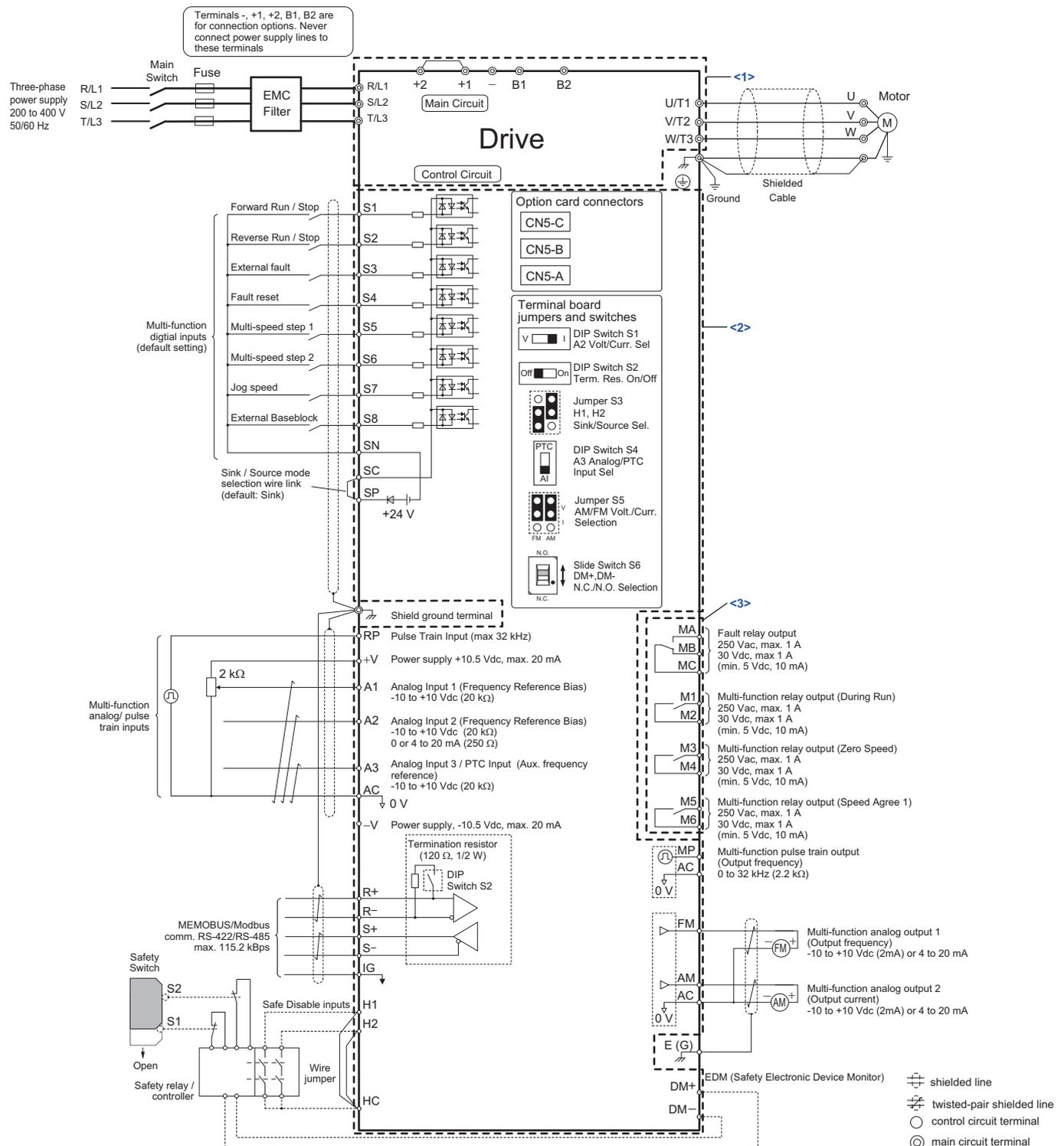
**Figure D.3 Wiring Diagram for CE Low Voltage Directive Compliance (example: 200 V Class)**
