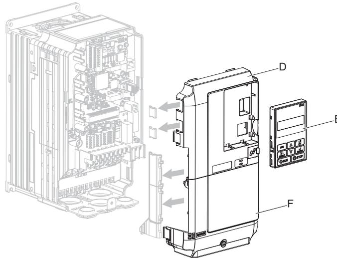
**Figure 8.15 Replace the Front Covers and Digital Operator**
