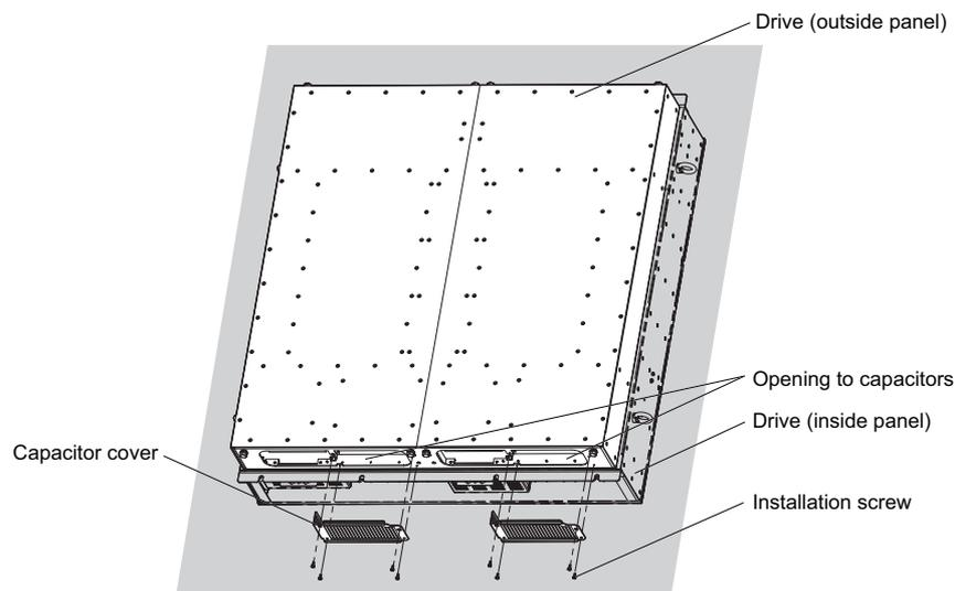
**Figure D.12 Capacitor Cover (4A0930, 4A1200)**
