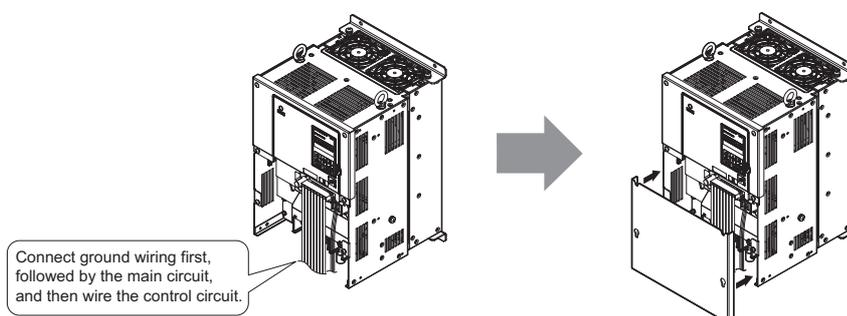
Figure 3.8 Reattaching the Terminal Cover on an IP00 Enclosure Drive
