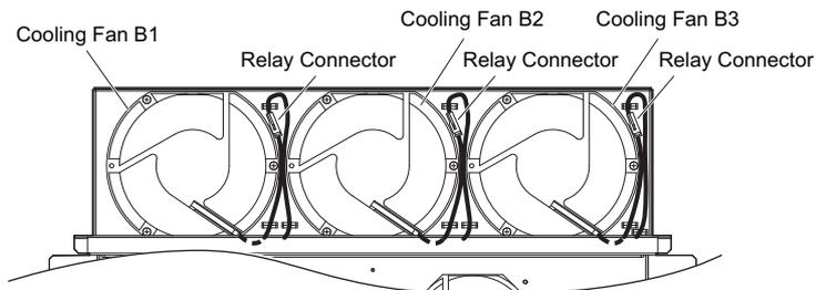
Figure 7.36 Cooling Fan Wiring: 4A0515 and 4A0675
