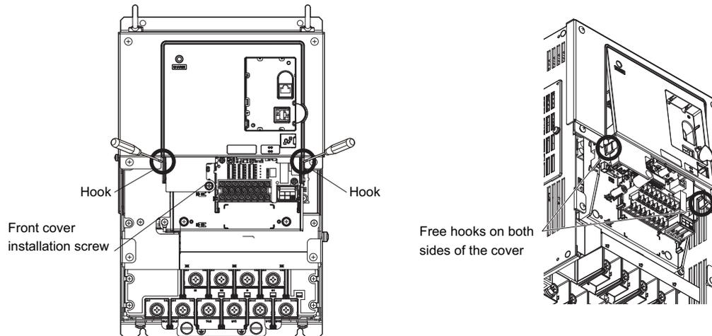
Figure 3.12 Remove the Front Cover (2A0110 to 2A0415 and 4A0058 to 4A1200)
