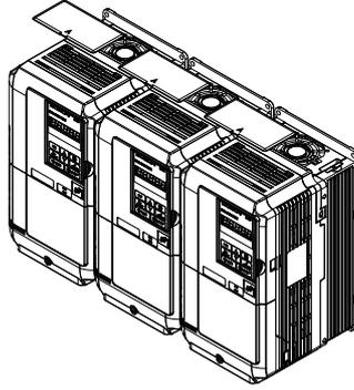
Figure 2.4 IP20/UL Type 1 Side-by-Side Mounting in Enclosure
