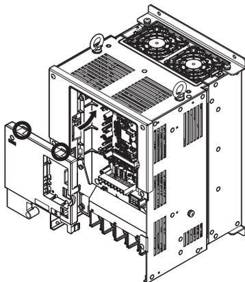
**Figure 3.14 Reattach the Front Cover (2A0110 to 2A0415 and 4A0058 to 4A1200)**
