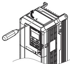
Figure 3.15 Removing the Top Protective Cover
