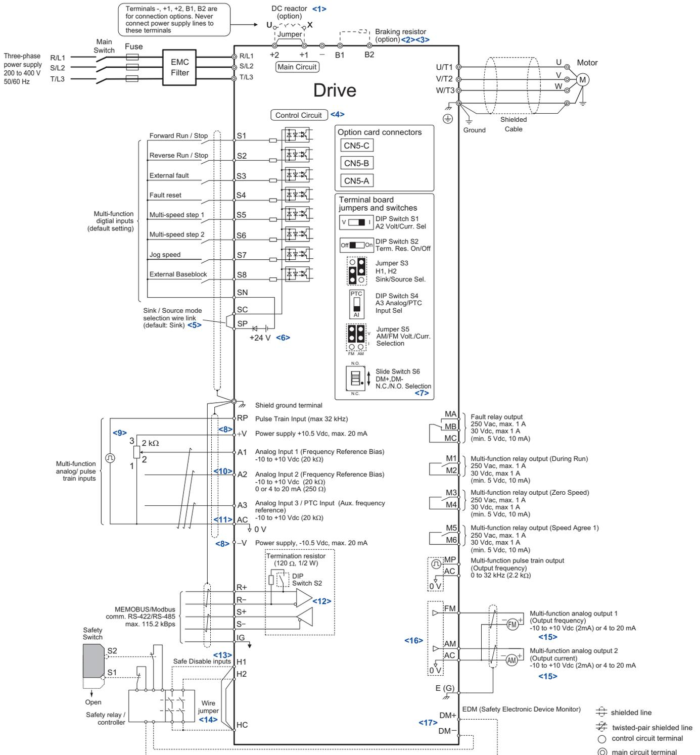
Figure 3.1 Drive Standard Connection Diagram (example: CIMR-A□2A0040)
