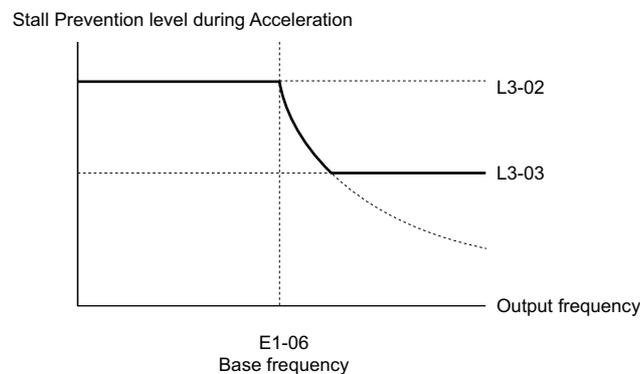
Figure 5.103 Stall Prevention Level and Limit During Acceleration
