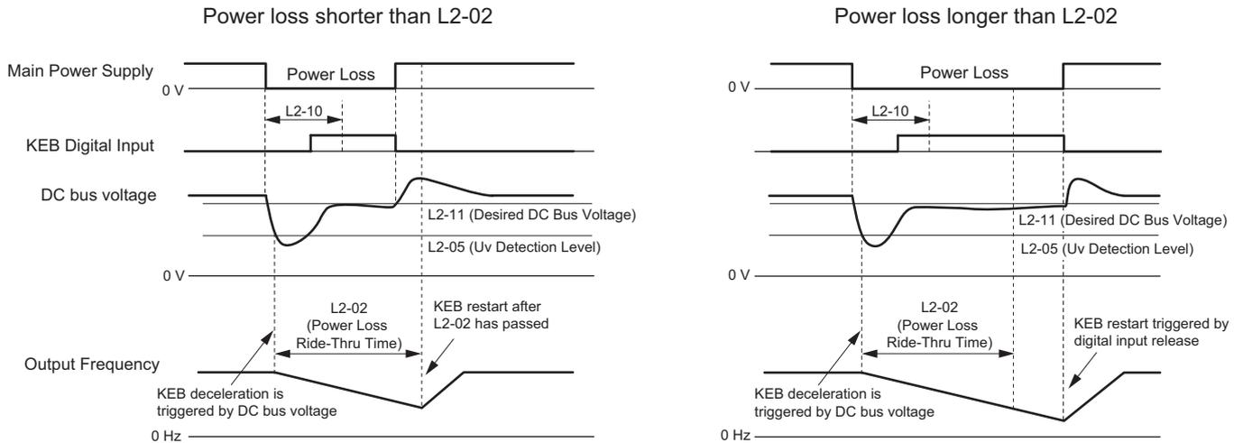
**Figure 5.97 KEB Operation Using L2-02 and KEB Input**
