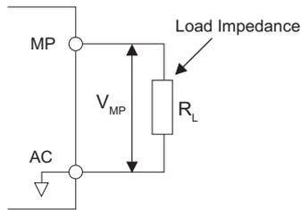
Figure 3.26 Pulse Output Connection Using Internal Voltage Supply
