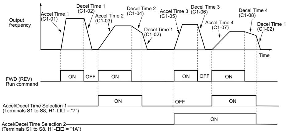
Figure 5.33 Timing Diagram of Accel/Decel Time Change
