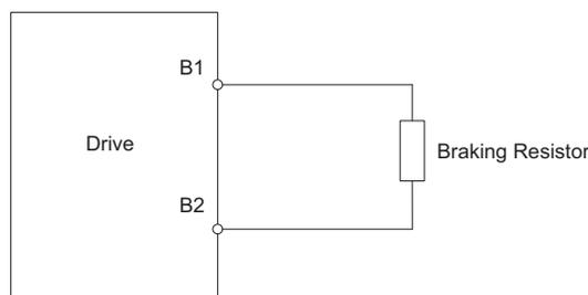
Figure 8.18 Connecting a Braking Resistor: ERF Type
