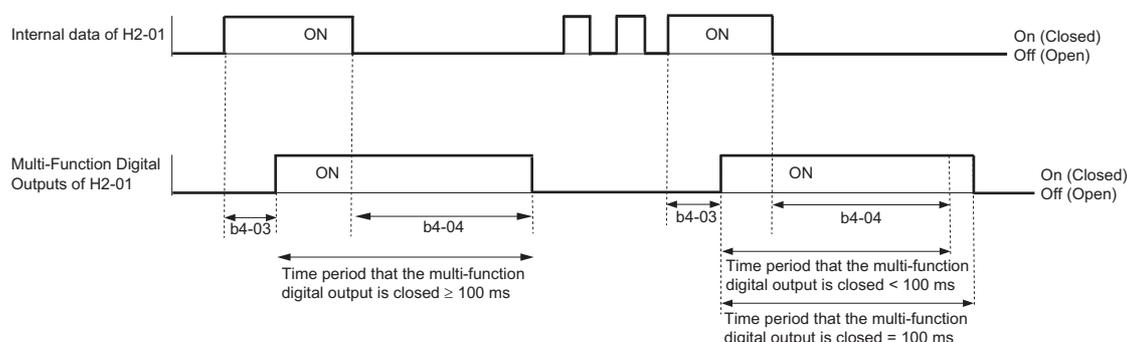
**Note:** Even if the length of the off-delay time and on-delay time for multi-function digital output are each less than 100 ms, the multi-function digital output closes for at least 100 ms.
