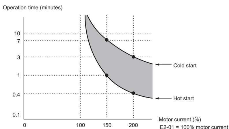
**Figure D.10 Motor Overload Protection Time**
