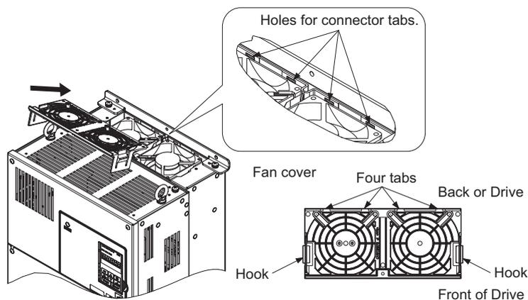
**Figure 7.18 Reattach the Fan Cover: 4A0088 and 4A0103**
