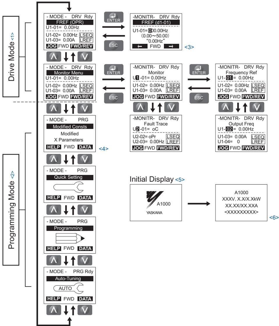
Figure 4.5 Digital Operator Menu and Screen Structure
