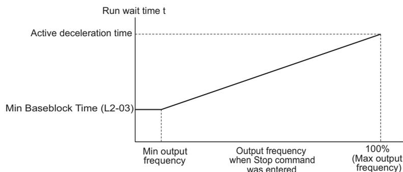
Figure 5.10 Run Wait Time Depending on Output Frequency
