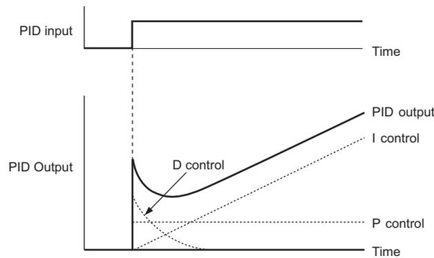
Figure 5.25 PID Operation
