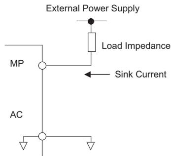
Figure 3.27 Pulse Output Connection Using External Voltage Supply
