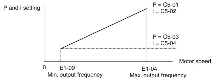
Figure 5.40 ASR Gain and Integral Time in V/fw/PG
