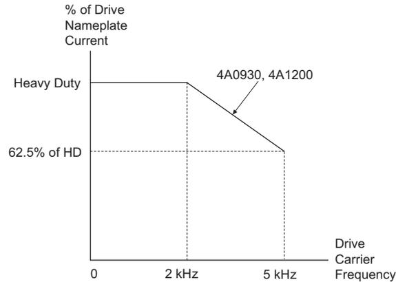
Figure A.6 Carrier Frequency Derating (CIMR-A□4A0930 and 4A1200)
