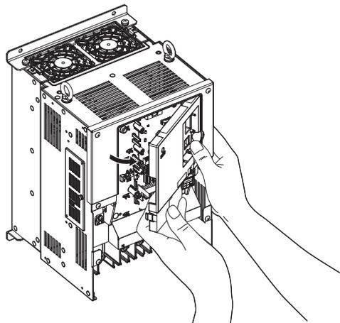
Figure 3.13 Remove the Front Cover (2A0110 to 2A0415 and 4A0058 to 4A1200)
