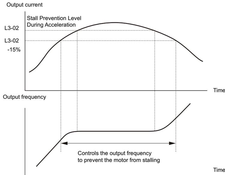
**Figure 5.101 Stall Prevention During Acceleration for Induction Motors**
