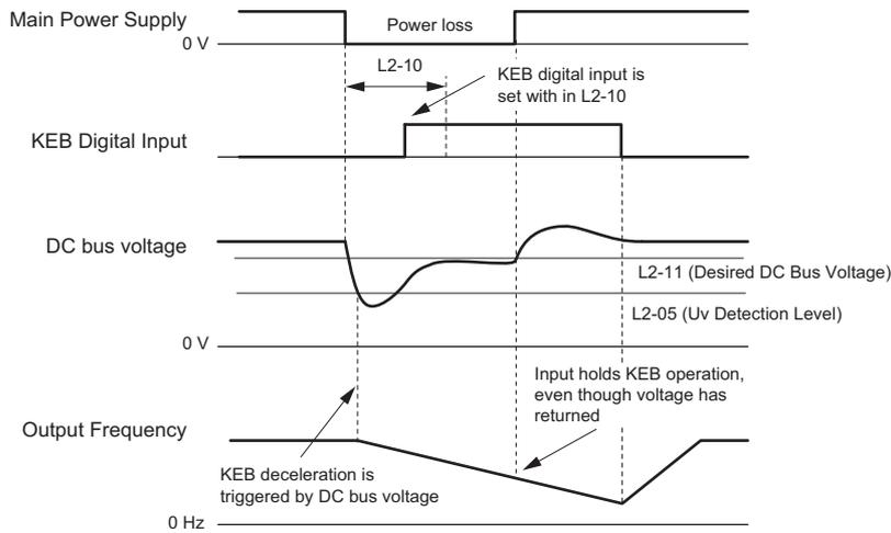
Figure 5.95 KEB Operation Using a KEB Input
