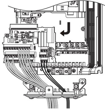
Figure 7.59 Drive Replacement: Remove the Terminal Board
