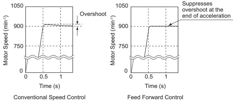
Figure 5.110 Overshoot Suppression by Feed Forward Control
