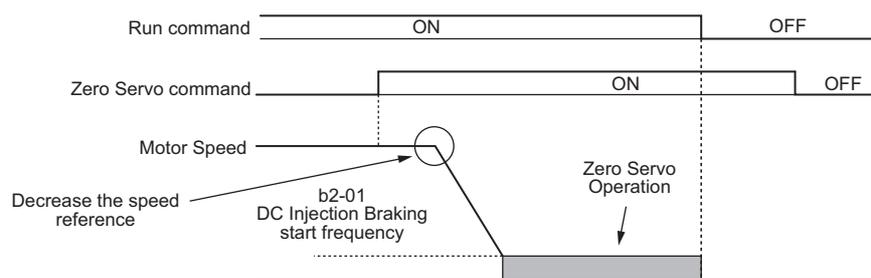
**Figure 5.32 Zero Servo Operation**
