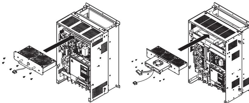
Figure 7.26 Installing the Cooling Fan Unit: 2A0169 to 2A0415, 4A0139 to 4A0362
