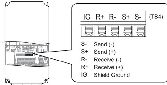
**Figure C.2 Serial Communications Cable Connection Terminals (TB4)**
