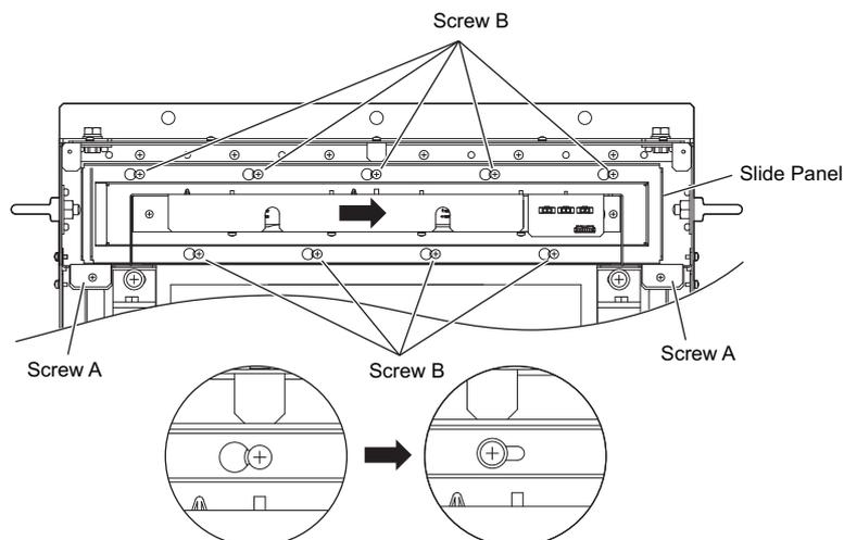
**Figure 7.33 Removing the Fan Unit: 4A0515 and 4A0675**
