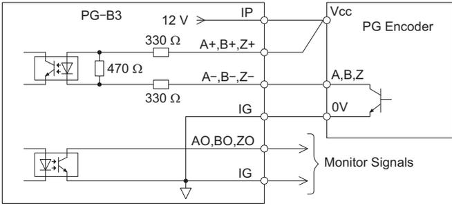
Figure 8.10 Open-Collector Outputs for the Interface Circuit
