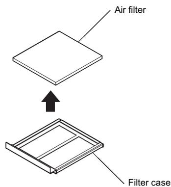
**Figure 7.55 Air Filter Replacement: Taking Out the Filter**
