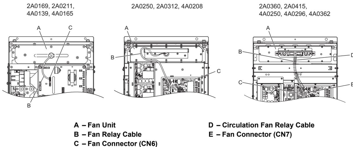
Figure 7.20 Cooling Fan Replacement: Fan Unit and Connectors
