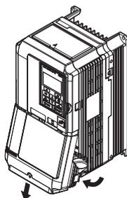
Figure 3.4 Removing the Terminal Cover on an IP20/UL Type 1 Enclosure Drive
