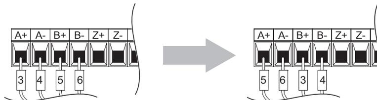
**Figure 8.17 A Channel and B Channel Wire Switching**
