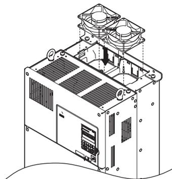
**Figure 7.16 Installing the Cooling Fan: 4A0088 and 4A0103**
