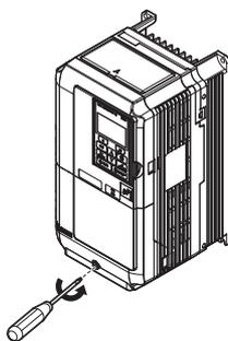
Figure 3.3 Removing the Terminal Cover on an IP20/UL Type 1 Enclosure Drive
