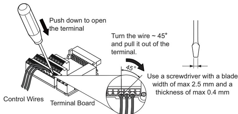
**Figure 3.23 Removing Wires from the Terminal Board**
