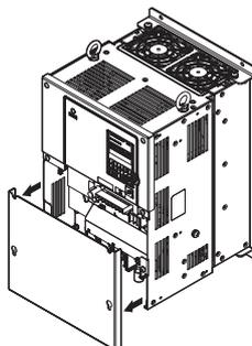
Figure 3.7 Removing the Terminal Cover on an IP00 Enclosure Drive
