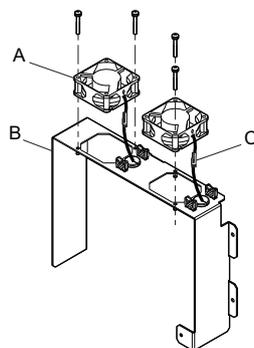
A – Circuit Board Cooling Fan                      C – Relay Connector
