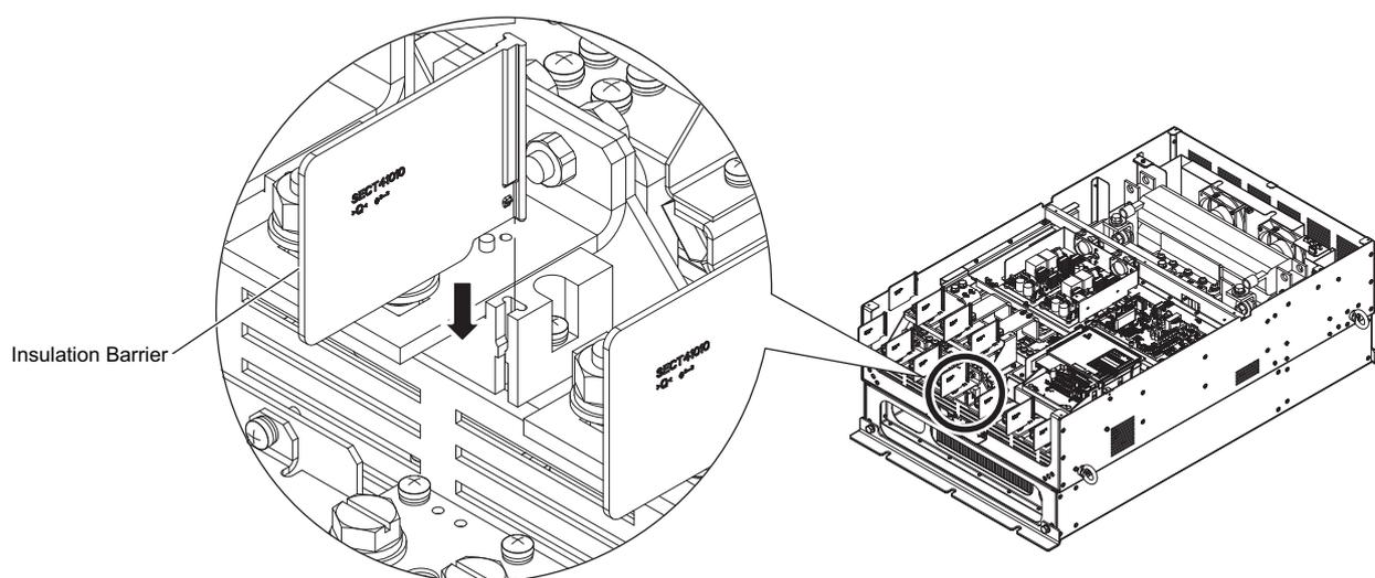
Figure 3.17 Installing insulation barriers
