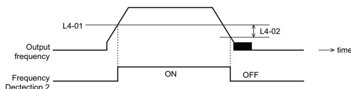
**Figure 4.12 Frequency Detection 2**
