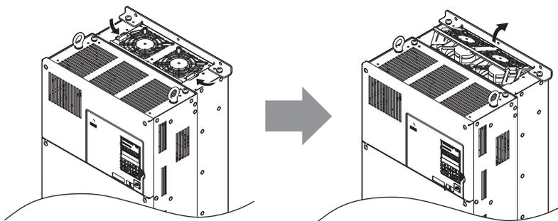
Figure 7.14 Removing the Cooling Fan Cover: 4A0088 and 4A0103
