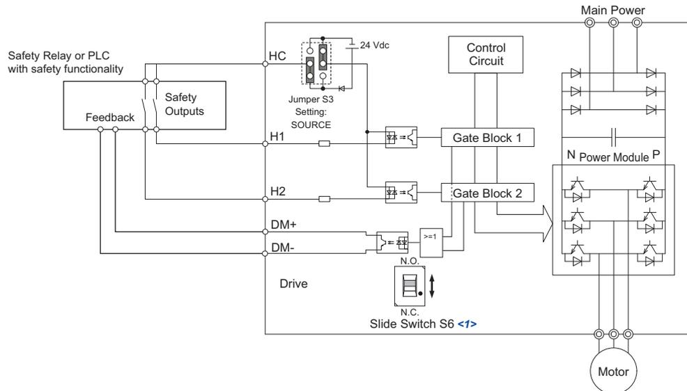
Figure D.13 Safe Disable Function Wiring Example (Source Mode)
