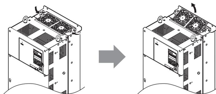
Figure 7.8 Removing the Cooling Fan Cover: 2A0110 and 2A0138, 4A0058 and 4A0072
