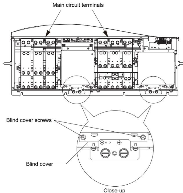
Figure 7.52 Air Filter Replacement: Removing the Blind Cover
