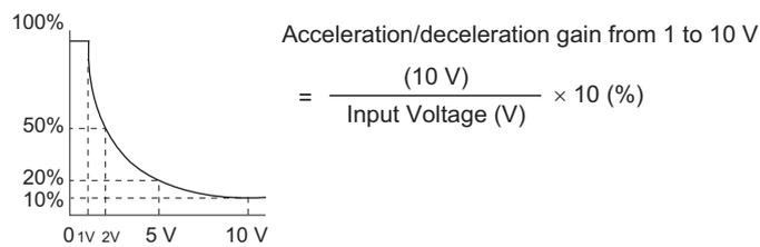
**Figure 5.83 Accel/Decel Time Gain with Analog Input Terminal**
