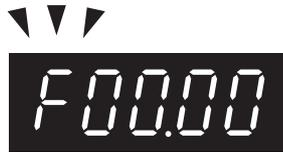
Figure 5.112 Ready for Setting Frequency Reference
