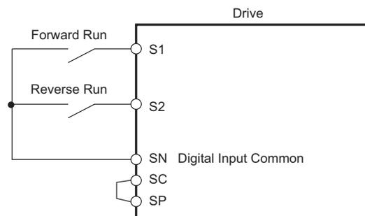
Figure 5.66 Example Wiring Diagram for 2-Wire Sequence
